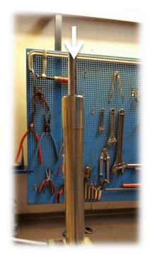
Press down the piston rod until the stop. If air was caught, the downwards resistance changes when the air is released.
