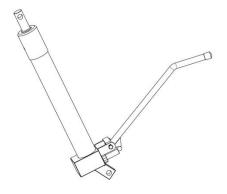
In very rear cases, the pumpcylinder still contains air and is malfunctioning.
