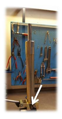
Open the release handle to allow the oilflow to go back and the piston rod to go down.
