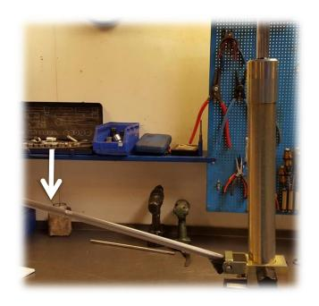
Pump the handle five times with the release handle at open position to ensure that the venting is complete. Close the release handle and the pumpcylinder is ready for use
