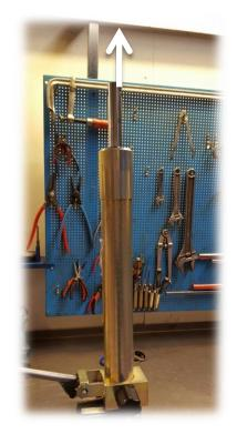
Open the release handle and press the piston rod upwards. If the pumpcylinder contains air the upwards resistance will change.
